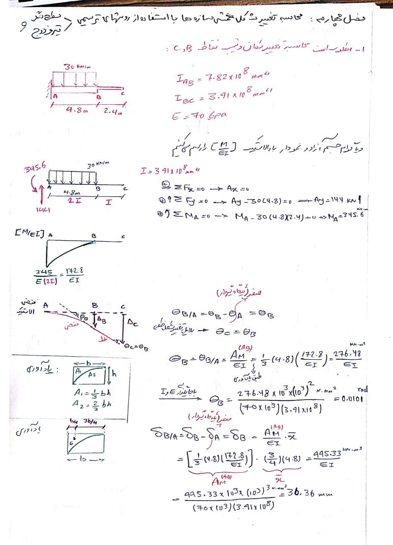
$$S_{C} = S_{C} - S_{A} = S_{C} = \frac{A_{M}^{(A_{C})}}{E_{I}} \cdot \Re = \left[\frac{1}{3}(4.8)\left(\frac{172.8}{E_{I}}\right)\right] \left(\frac{3}{4}\times4.8 + 2.4\right) = \frac{1658.88}{E_{I}}$$
