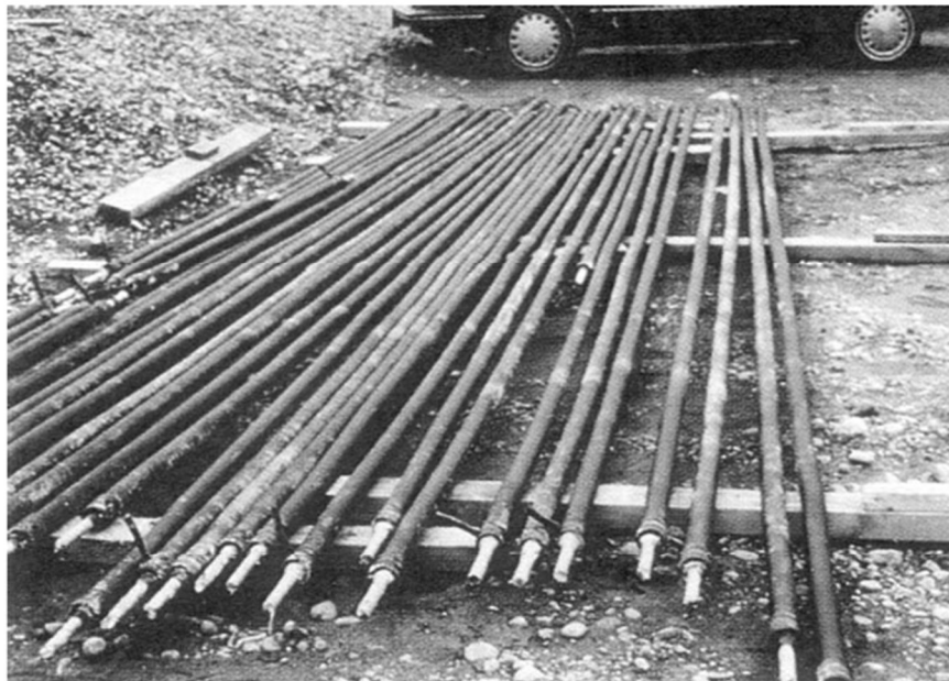
Figure 4.4: Nail Bars (in light color at end of nails) Encapsulated by Sheathing (dark color) Prior to Nail Installation.
