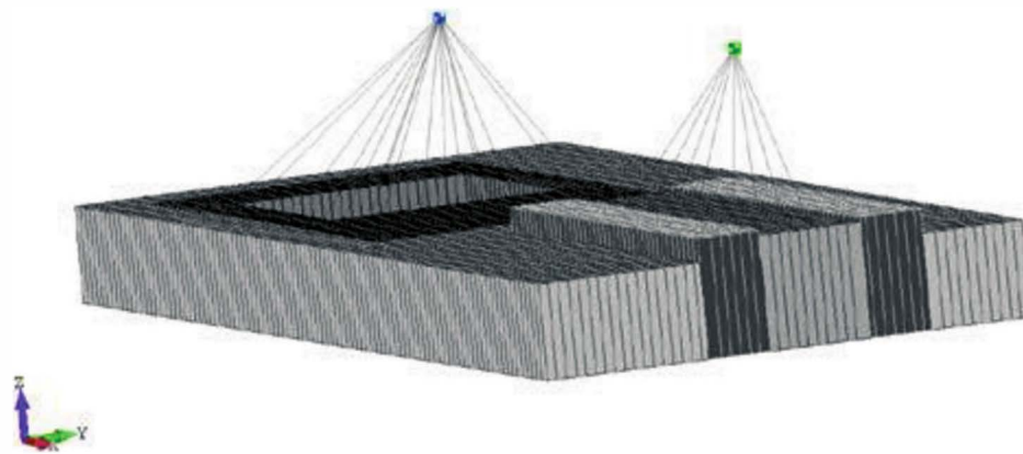
Fig. 6.3.3.3—Finite element model of inertia block and machine (image courtesy of GERB Vibration Control Systems, Inc.).
